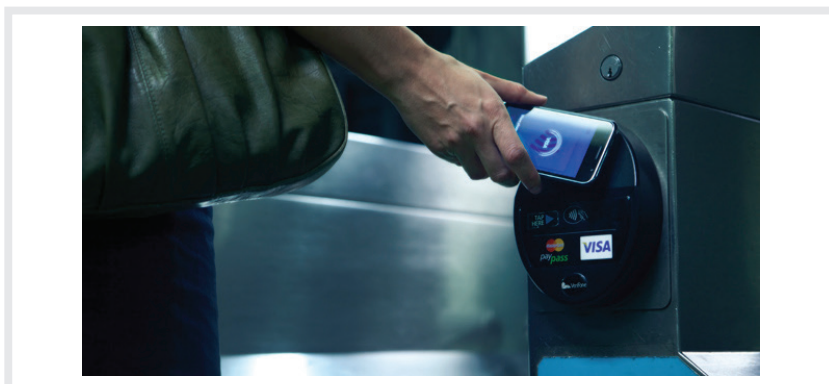
Figure 11. Using a mobile phone to make an NFC payment. (Jargon Media, 2011)
